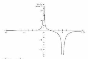
e) For  $x >> a: V \approx \frac{-kqx}{x^2} = \frac{-kq}{x}$ , which is the same as the potential of a point charge -q. (Note: The two charges must be added with the correct sign.)
